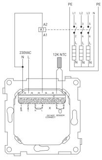
K1: contactor with integral supression device
